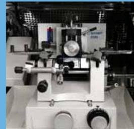
The Bright 5040 microtome is based on original and proven designs that can cope with high cutting loads and yet perform very favourably under conditions of low temperature. Based on the principle of a parallelogram of forces, the 5040 is of unique
